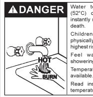
Water temperature over 125°F (52°C) can cause severe burns instantly resulting in severe injury or death.
